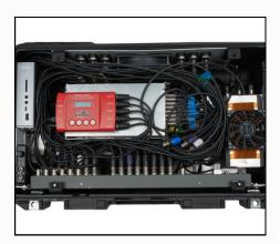
Includes a custom enclosure to accommodate a single lane capture card on the upper shelf (for example, Black Magic Deck Link Quad 2 or Duo 2).
