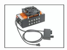
The power distribution box allows for seamless power swap between the 24V primary & secondary power inputs. The regulated 20V side powers either the CalDigit TS4+ or TS3+ to power your Macbook Pro laptop. It charges the MacBook Pro up to 86 watts via TS3 and 98 watts via TS4. Regulated 12volt power distribution system powers up to 10 devices via 2pin Lemo 0B ports (up to 3amps). Total shared load is 12 Amps (144 Watts).
