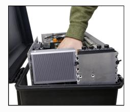
Loosen and pull out internal frame to access components when needed.
