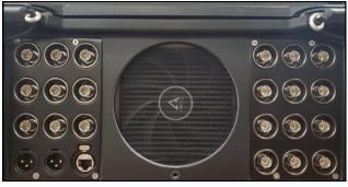
BNC label plates provide a flat surface for labelling connectors.
