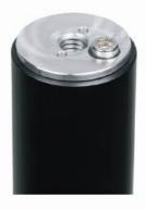
To remove Jam Plug, use 4mm or 5/32 hex key too loosen M5 SHCS until the screw head is protruding out of the counterbored hole. Whack the top of the SHCS to loosen the jam plug for removal.
